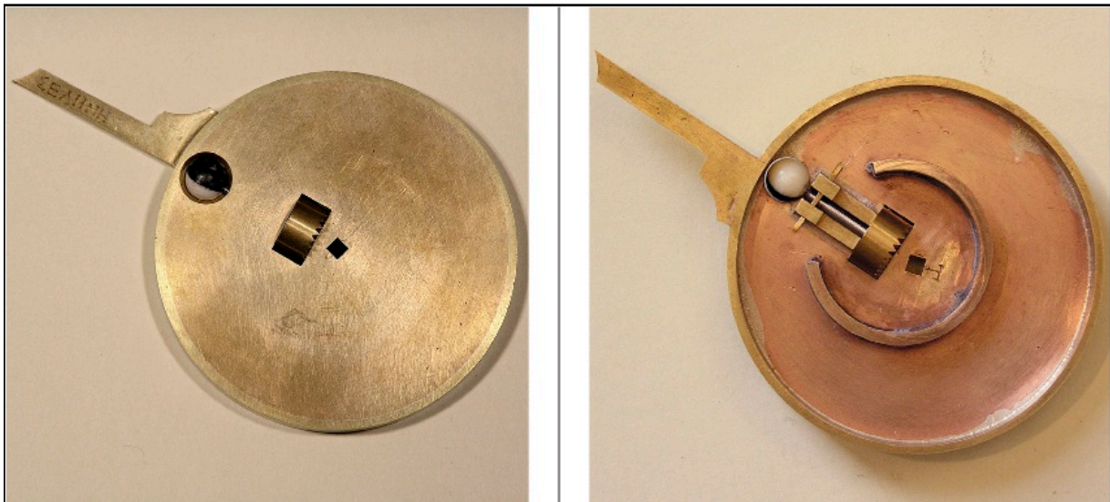
Fig. 37: Wright's reconstruction for the Moon phase display (Wright, 2006a)
