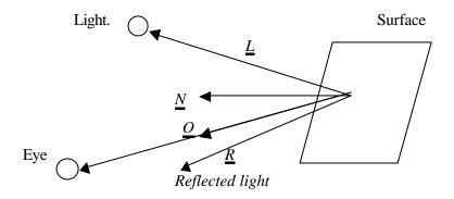
If <u>N</u> is a unit normal then we can show that  $\underline{R} = 2(\underline{N} \cdot \underline{L})\underline{N} - \underline{L}$ . The component of reflected light is  $(\underline{O},\underline{R})\underline{O}$  if <u>O</u> is a unit vector in the direction of the observer. Scaling factors on the length of this vector can then be used to generate the desired effect. Spot lights from the observer that can be turned on and off (a torch) are used to good effect in some game play.
